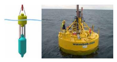
The point absorber is a floating structure that captures energy from the vertical motion of the waves. This up-and-down motion of the device drives generators that create an electric current.
