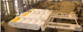
This style of device harnesses wave energy directly from the surging and swelling motion of waves. It uses the oscillation between a float, flap, or membrane and a fixed point. That movement creates a usable form of mechanical energy. Similar devices are also being developed that utilize pitching, heaving, and swaying motions.
