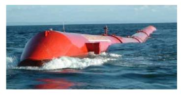
This device is long and multi-segmented and floats on the surface. The attenuator is anchored in place with a mooring line and positioned perpendicularly to incoming waves. Some attenuators tap only the heave (vertical motion); others tap both heave and surge. The device captures energy as the motion of the wave causes it to flex where the segments connect. This movement then drives hydraulic pumps or generators.
