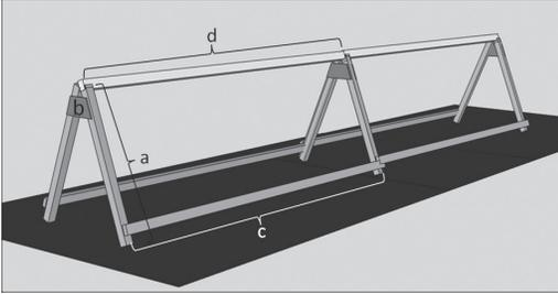
**Figure 2.** Detail of the above-ground tunnel structure prior to the attachment of the plywood sheets. A-frames were constructed with (a) 1.2-m sections of 50.8 x 50.8-mm lumber joined at the top with (b) a cut piece of 9.5-mm thick plywood. We connected consecutive A-frames with (c) 2.4-m lengths of 25.4 x 50.8-mm lumber approximately 76 mm from the bottom and (d) 50.8 x 50.8-mm lumber at the top.
