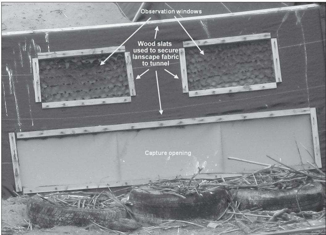
**Figure 3.** Detail of the completed above-ground tunnel.
