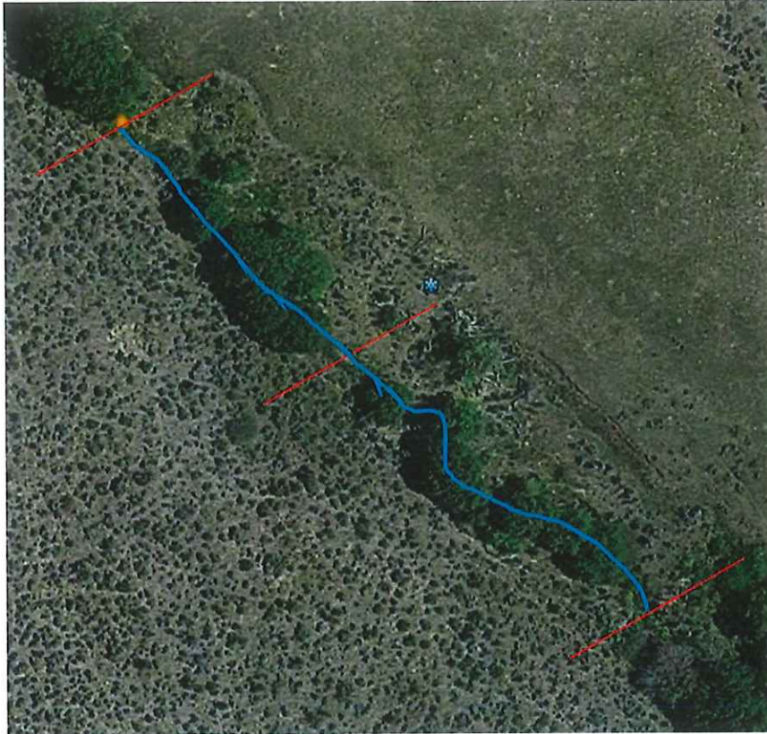
Schematic representing three transects for measuring stream morphology and riparian-upland vegetation. Also shows a 330-ft reach for measuring riparian vegetation using the 'greenline' method.
